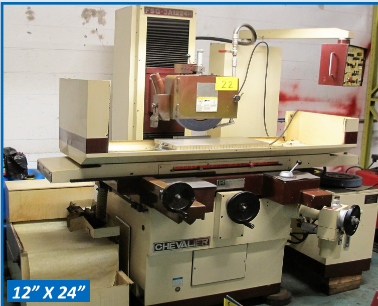
CHEVALIER FSG-3A1224H AUTO HYDRAULIC SURFACE GRINDER
